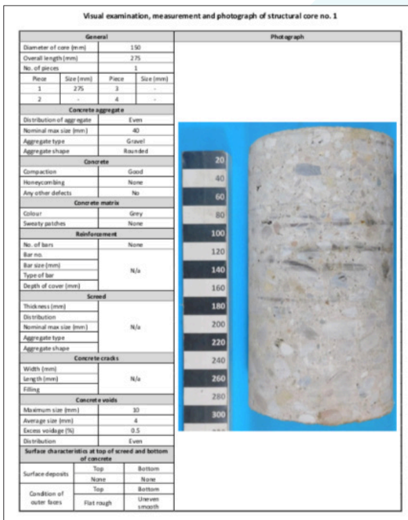
Diagrams show a typical coring report and DCP / CBR profile
